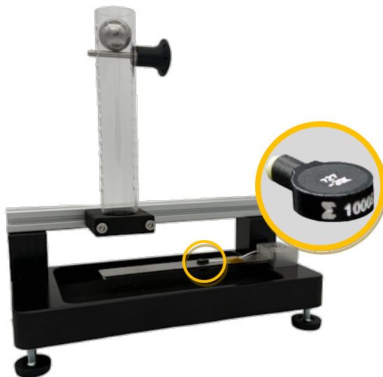
"Ball Drop" Fixture Instrumented With PR Accel
