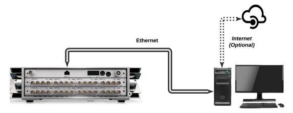
By default, the network adapters in MECALC mainframes obtain an IP from the client's <u>DHCP</u> server. In the diagram above, there is no DHCP server available. Consequently, the mainframe's ethernet adapter will auto-assign its IP address (<u>APIPA</u>) in the range of 169.254.1.0 through 169.254.255 with a subnet mask of 255.255.0.0.
