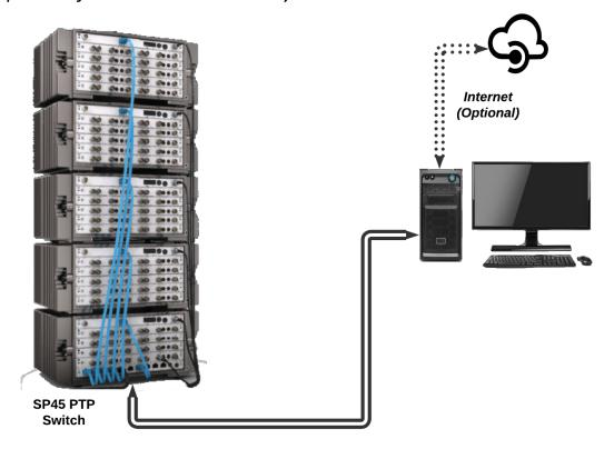
Multiple mainframes are connected to MECALC's SP45 PTP switch (installed in any one of the mainframes). The SP-45 supports the <u>PTP</u> network protocol. Each mainframe is configured for PTP, ensuring that clocks on all modules are synchronized for alignment of channel data. The PC connects to one of the open ports of the SP-45 switch.
