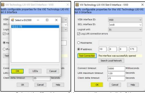
Select the IP address of the controller and click OK Test the connection and click OK
