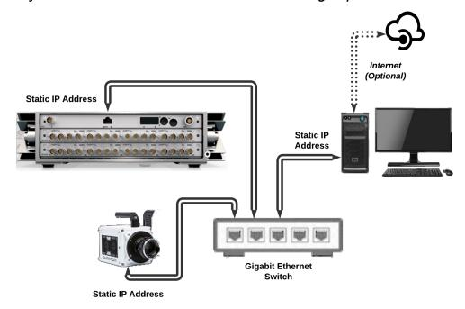
Tools and software provided by a camera manufacturer may require a LAN with a specific IP address range. In the diagram above, all ethernet adapters are configured with a static IP address and appropriate subnet mask. Additional ethernet-based devices (such as an LXI-VXI EX2500a controller) can be added to the LAN if assigned a static IP in the subnet range.
