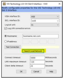
Click the button to Search Local Network For multiple controllers, assign a unique "Logical Unit" number to each controller
