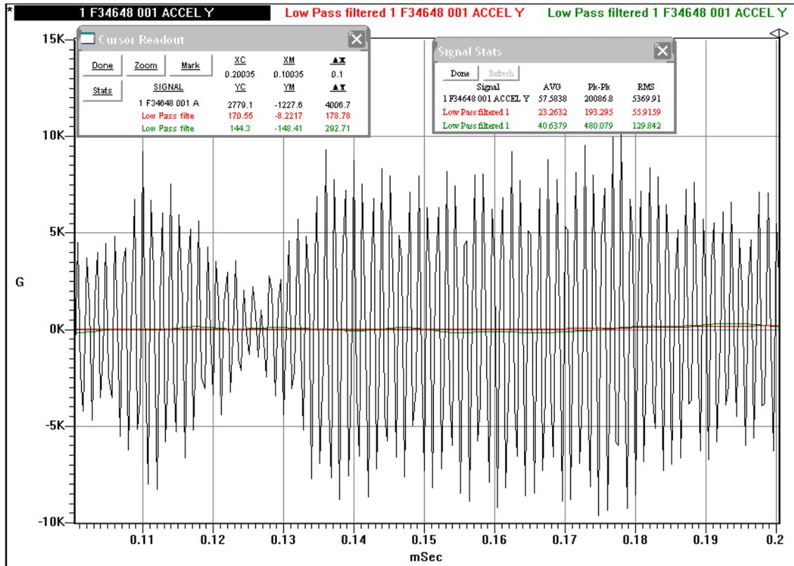
Figure 7c: A closer zoom showing broadband content. A slew rate limited amplifier will not present this waveform to the digitizing system.
