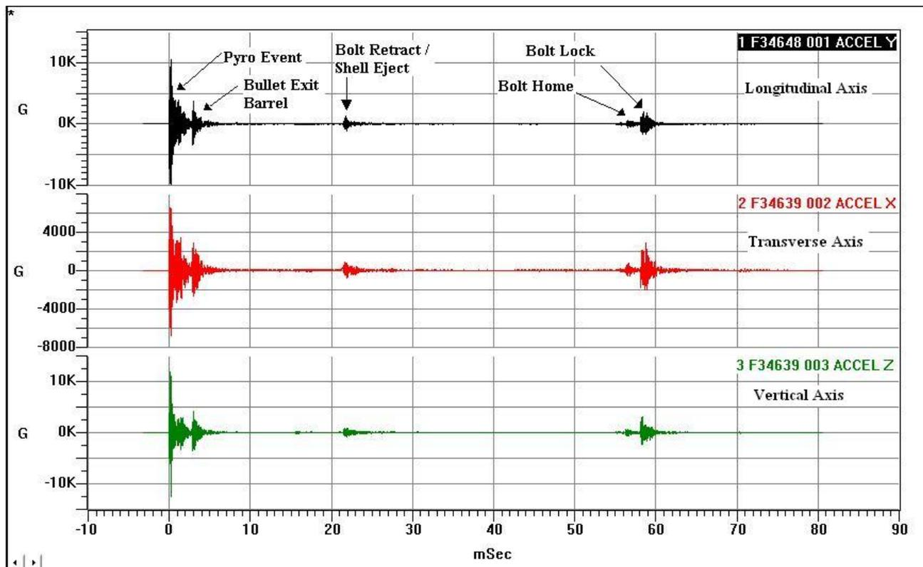
Figure 4: Broadband Data capture Single Fire Event X, Y, Z axis: Note G Levels ~10kG.
