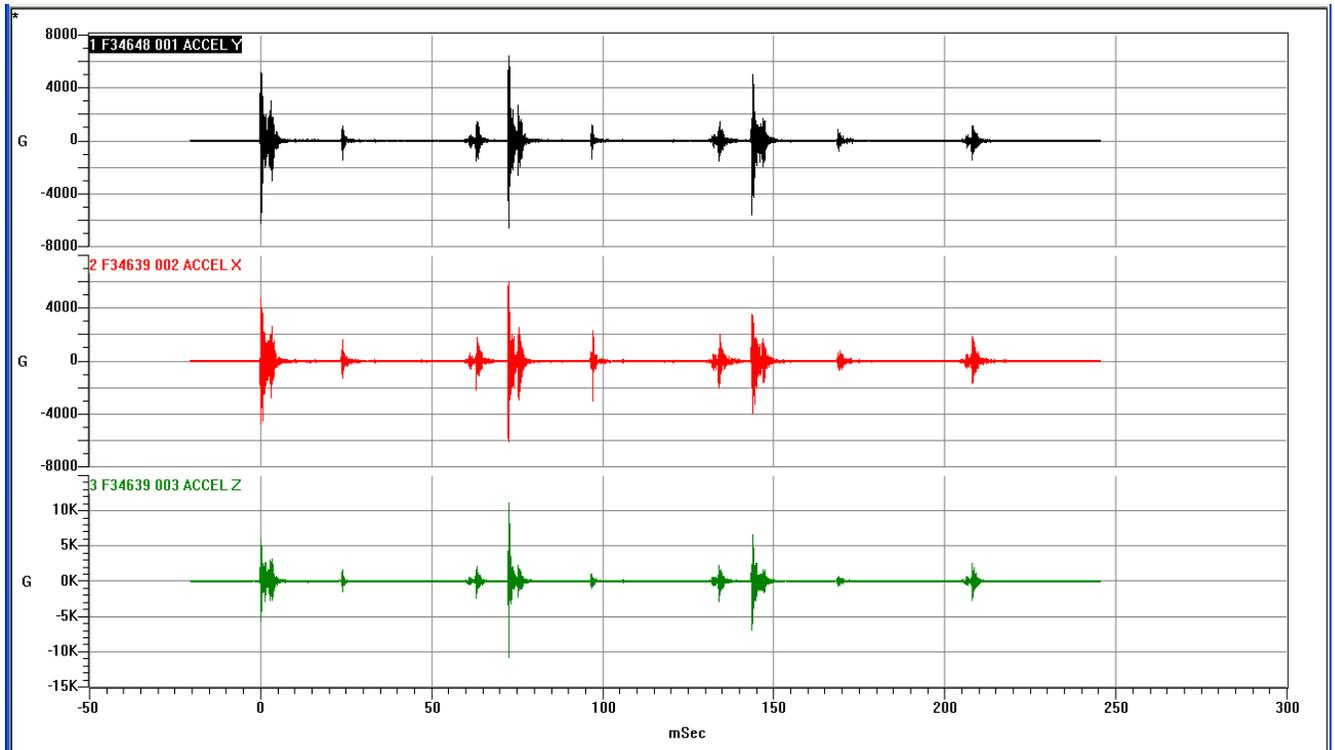
**Figure 11: Triaxial Acceleration Time History for three round burst in all three axes.
