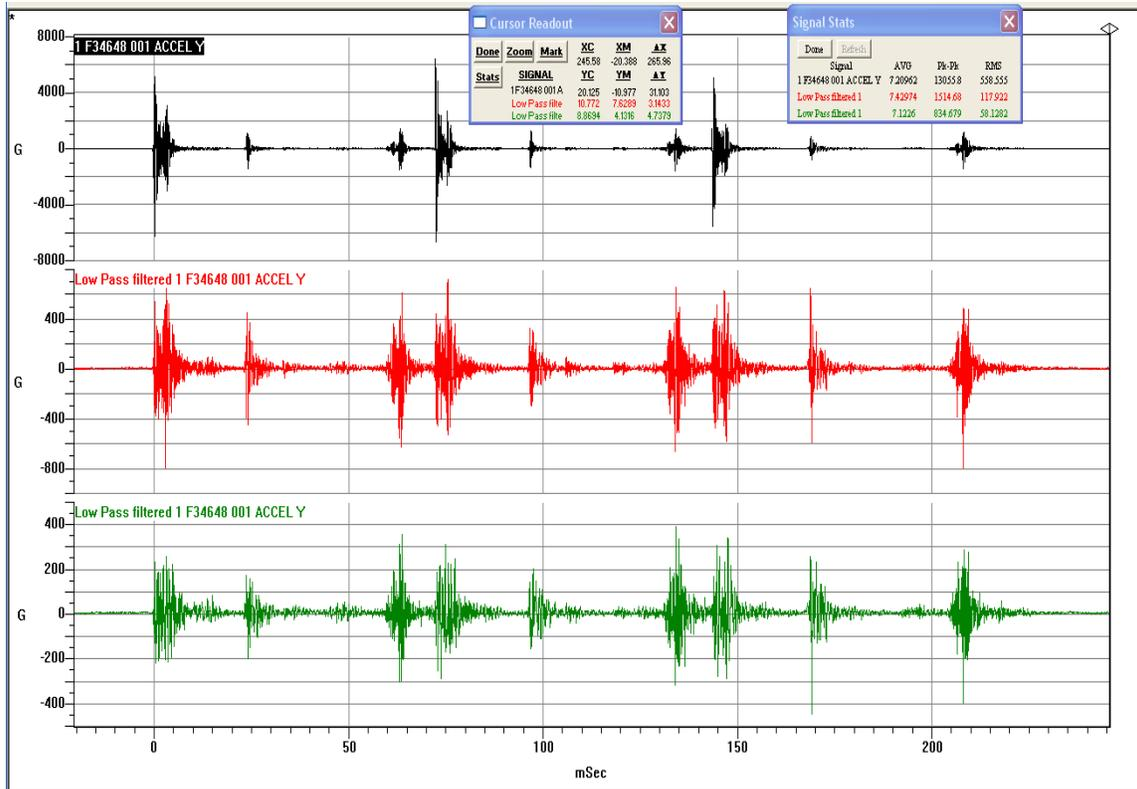
**Figure 15: Three Time History plots show the longitudinal axis only. (Black = Broadband, Red = 100 KHz, Green = 10 KHz)**
