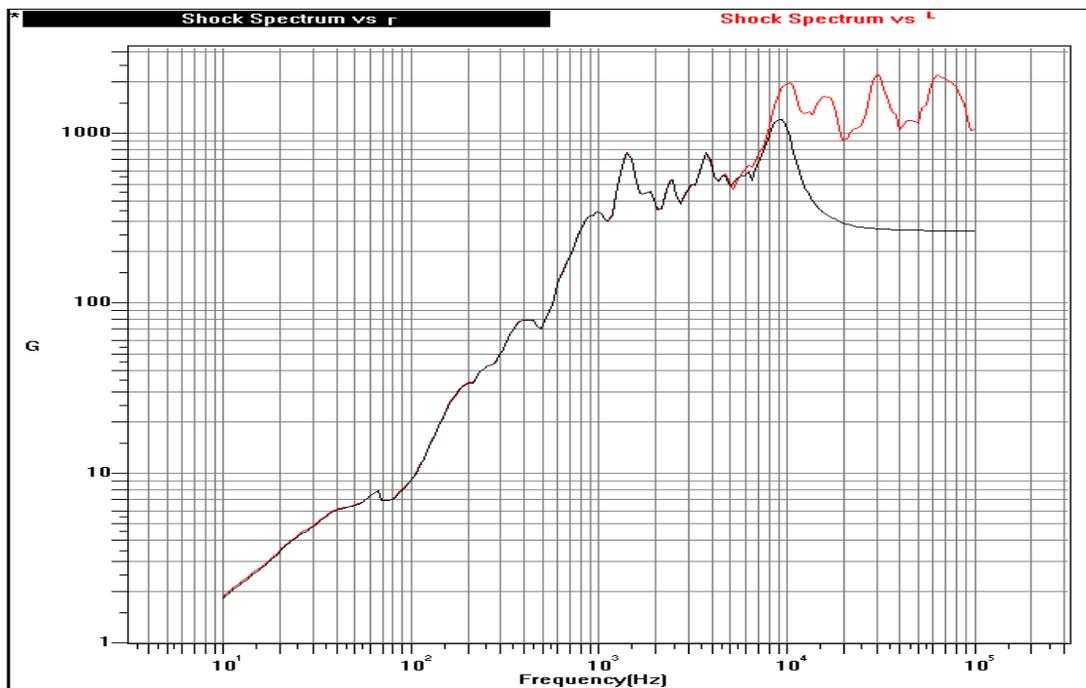
Figure 8: Y axis, SRS of Pyro-Segment, Digitally Filtered to 10 KHz (Black) and 100 KHz (Red) with Q=10.
