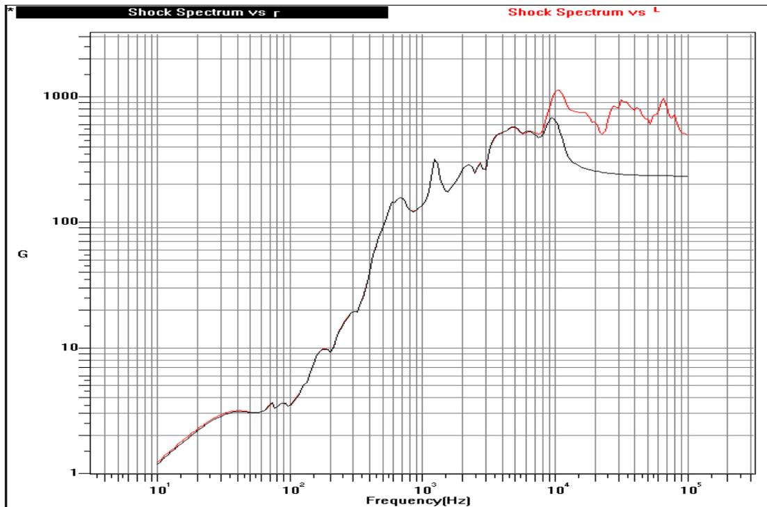
**Figure 9: Y axis, SRS of Retractor / Eject pulse-Segment, Digitally Filtered to 10 KHz (Black) and 100 KHz (Red) with Q=10.
