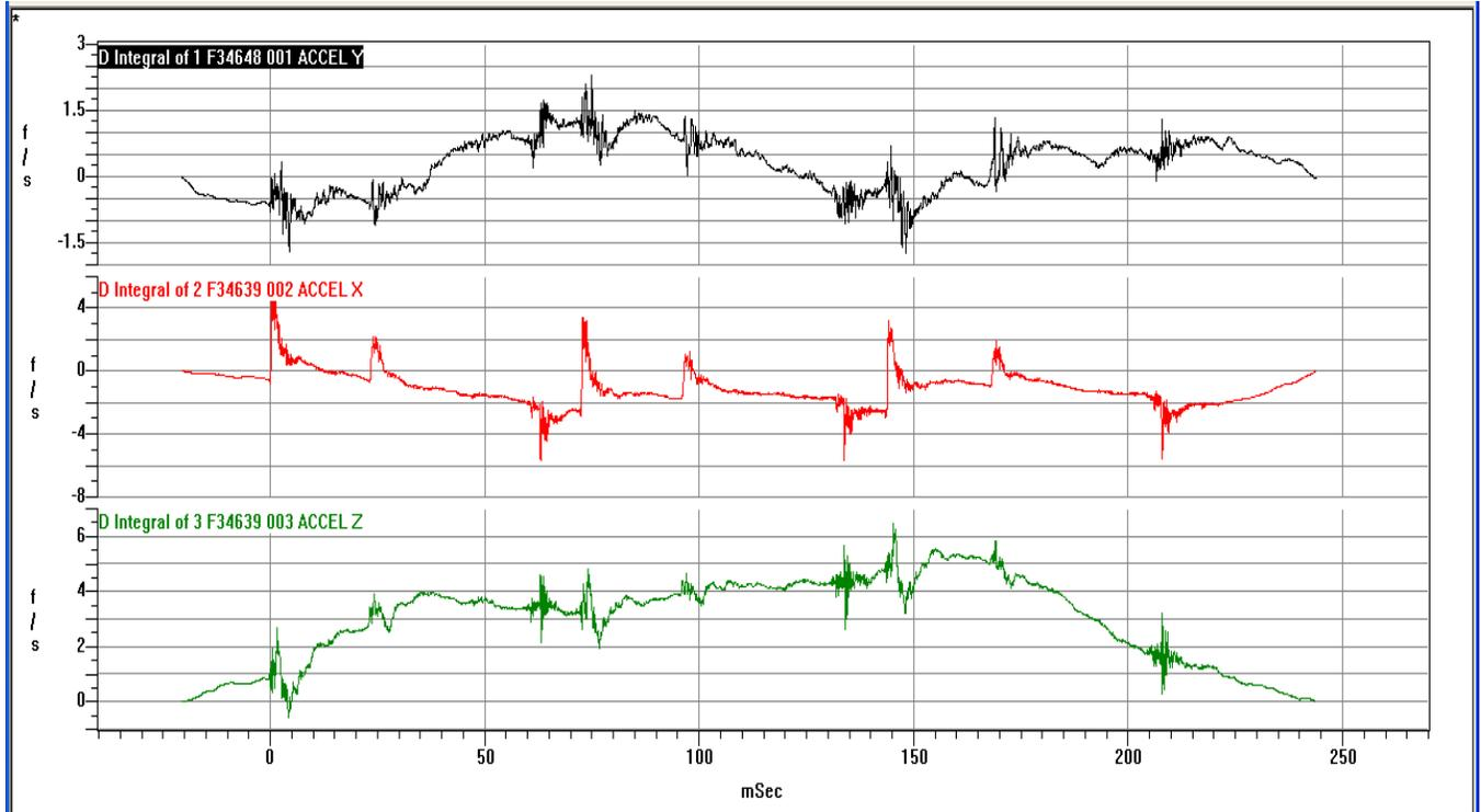
**Figure 12: Triaxial Velocity Time Histories for three round burst in all three axes.
