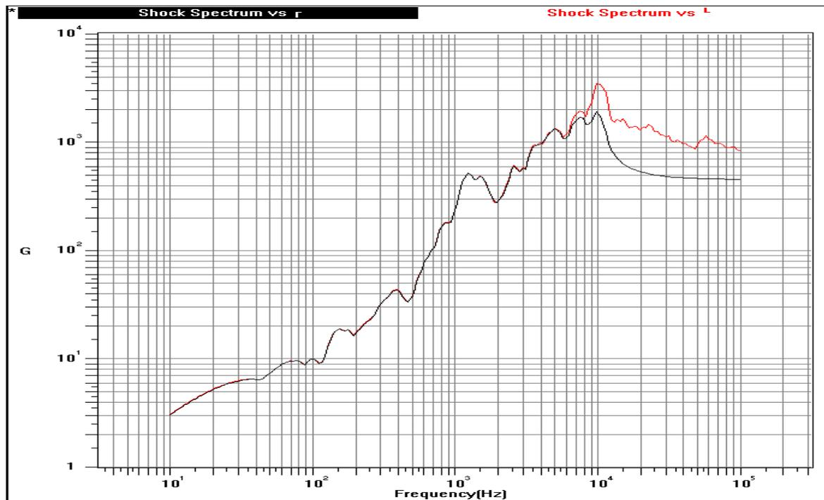
**Figure 10: Y axis, SRS of Bolt Home/Lock Pulse-Segment, Digitally Filtered to 10 KHz (Black) and 100 KHz (Red) with Q=10.**
