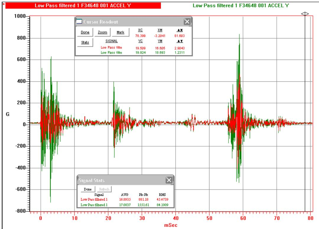
Figure 7a: Y-Axis Live Fire Event (from Figure 4) Filtered to 10 KHz (Red) and 100 KHz (Green).
