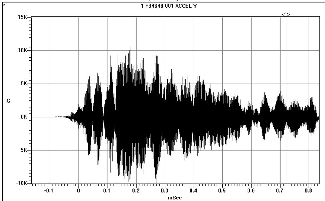
Figure 7b: A zoom of the time history of just the Y axis Pyroshock (first impulse) event showing ~20,000 g Peak-to-Peak content.
