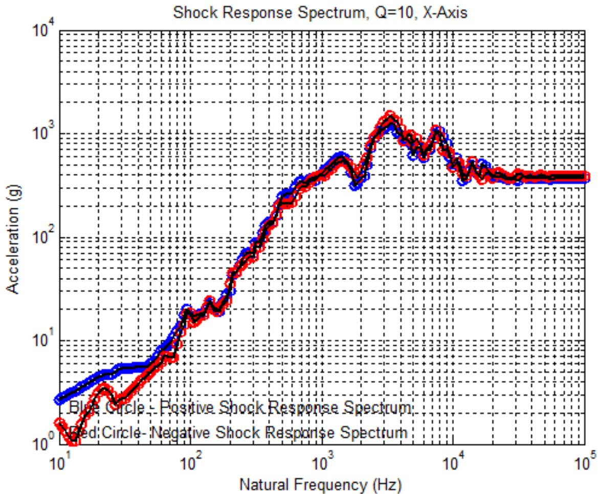
**Figure 3: Shock Response Spectra for Longitudinal Gunfire Shock in Figure 1.**
