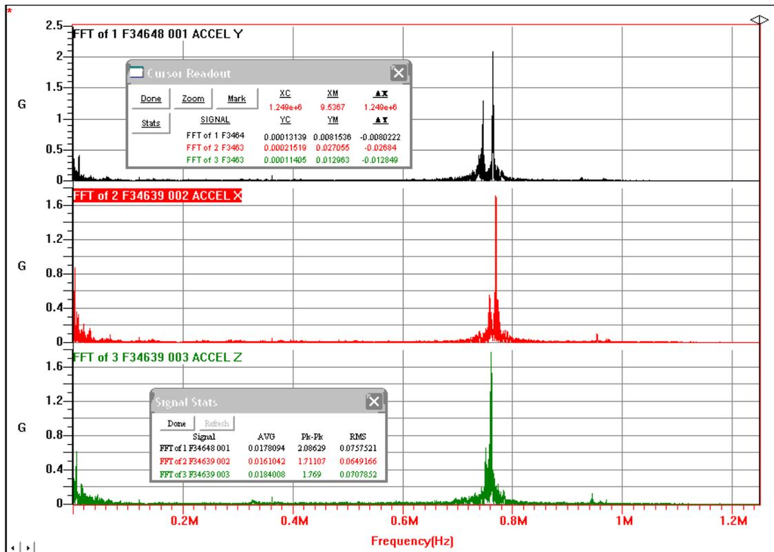
Figure 6: Discrete Fourier Transforms for Triaxial Data in Figure 3 Depicting the Significant Transducer Resonance at ~750 KHz in all 3 axes.
