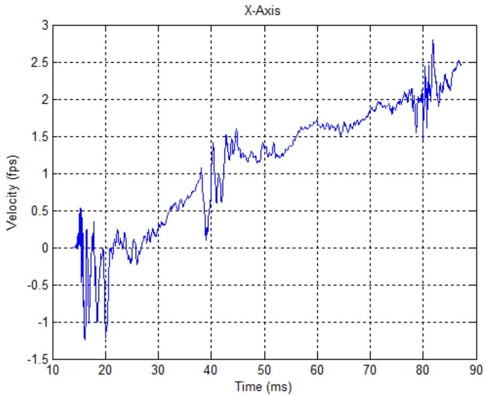
**Figure 2: Velocity for Longitudinal Gunfire Shock (Integral of Acceleration in Figure 1).**
