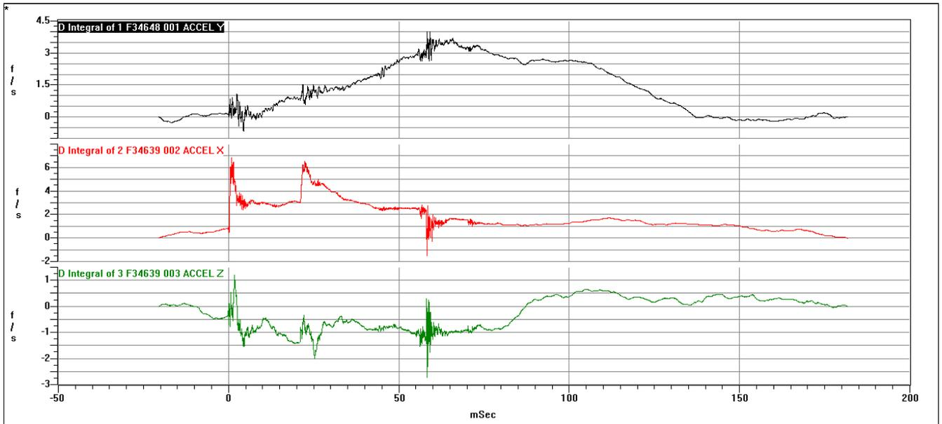
Figure 5: Velocity Time Histories (Integral of Acceleration Data in Figure 4).
