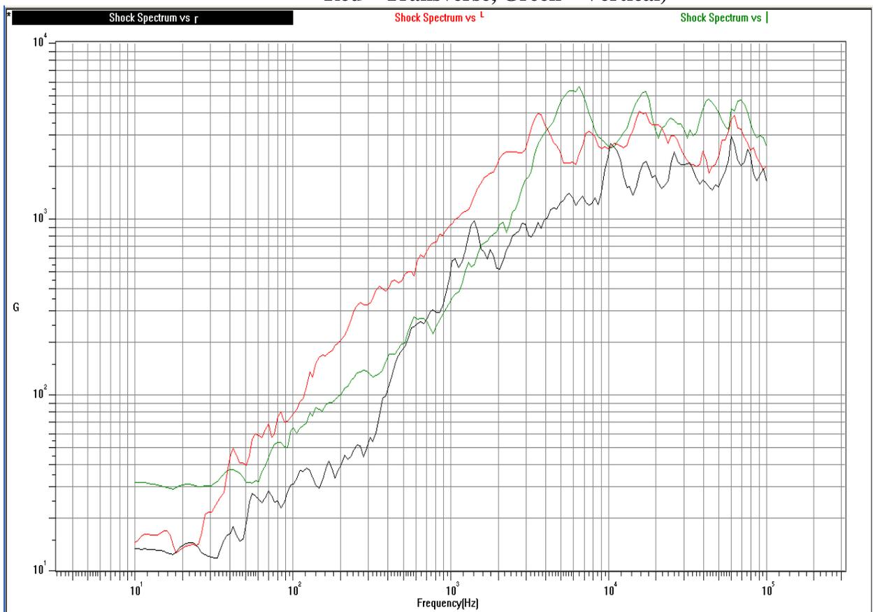
**Figure 14: Three Round Composite SRS for Acceleration Time History in Figure 11 (Black - Longitudinal, Red – Transverse, Green – Vertical with Q=10).**
