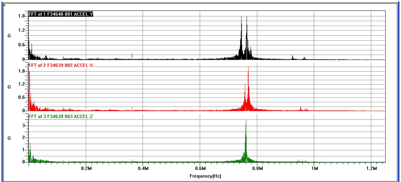
**Figure 13: Three Round Composite FFT for Triaxial Acceleration (Black - Longitudinal, Red – Transverse, Green – Vertical)**
